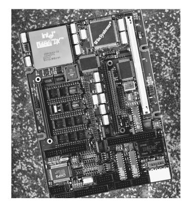
each with RS-232, and optional RS-422/485 levels, Centronics parallel I/O port, floppy disk controller, IDE hard disk interface, and 16-bit PC/104 expansion connector.
